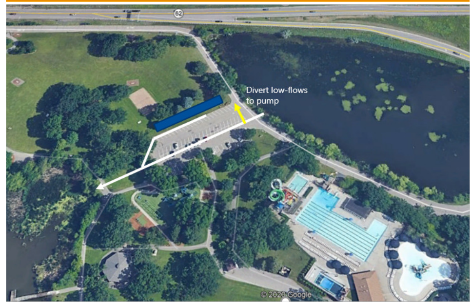
Alt Concept 2- divert low flows to pump/filtration BMP
