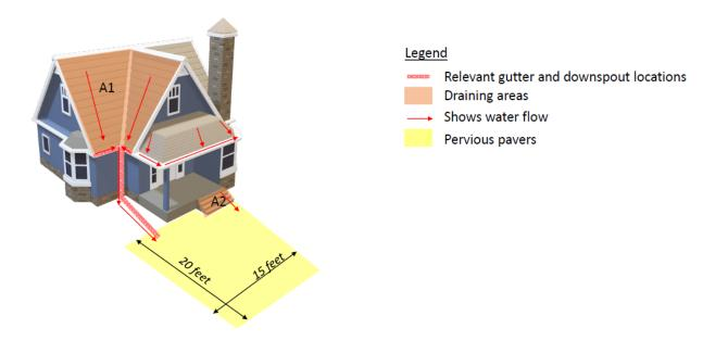
5. Fill in the table with information about the areas that drain to the pervious pavement system. *If you need information on how to calculate the square footage of the drainage areas, refer to "measuring on the map" in this guide for assistance.*
