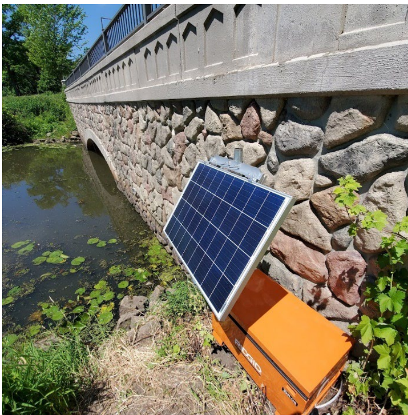
Figure 2: Picture of Normandale inlet PIT antenna monitoring station.
