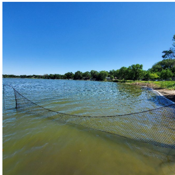
FIGURE 8: PHOTO SHOWING A BAITED BOX NET TRAP WITH WALLS RAISED.
