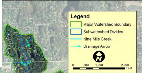
As visibly shown on the map, a lot of stormwater lead to Minnetoga Lake. These pipes carry water that fall on this part of the watershed and is not infiltrated in the ground. This water washes chemicals or pollutants left on lawns, streets, roof tops and parking lots and carries it right into Minnetoga Lake. This makes every curb part of a shoreline!
