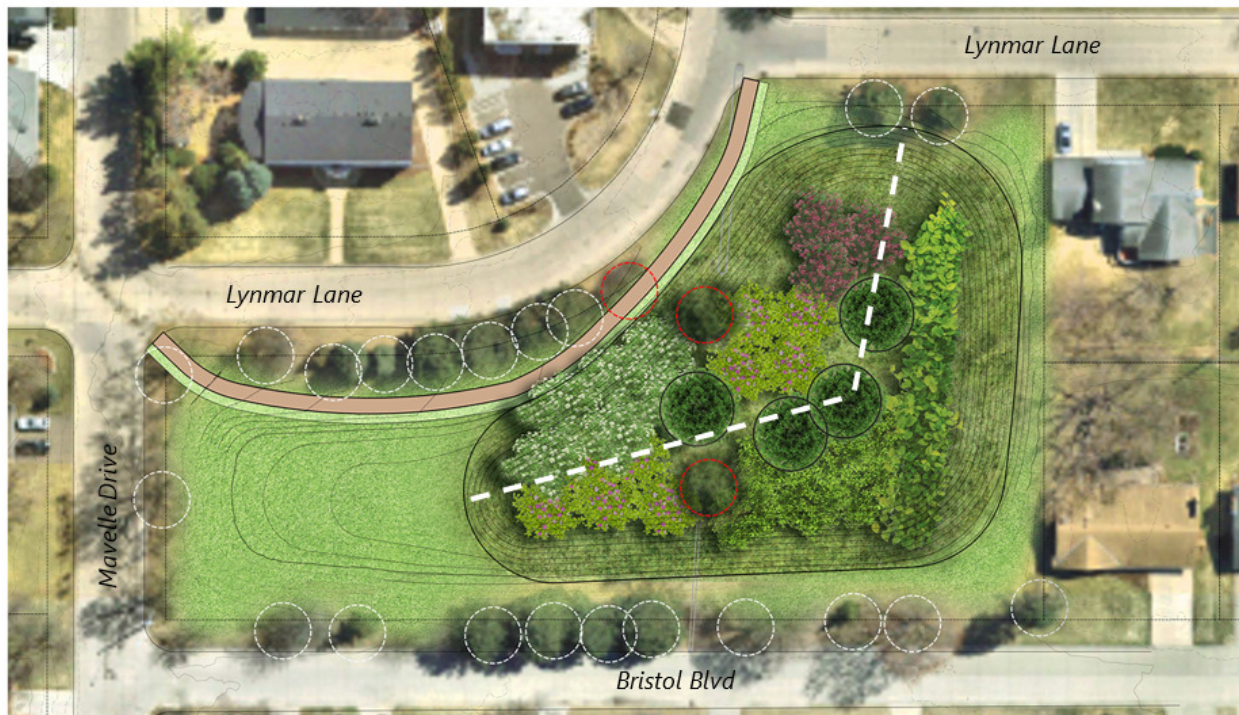
Figure 3-2. Lynmar Basin Stormwater Retrofit Conceptual Design with sand trenches (dashed white line)
