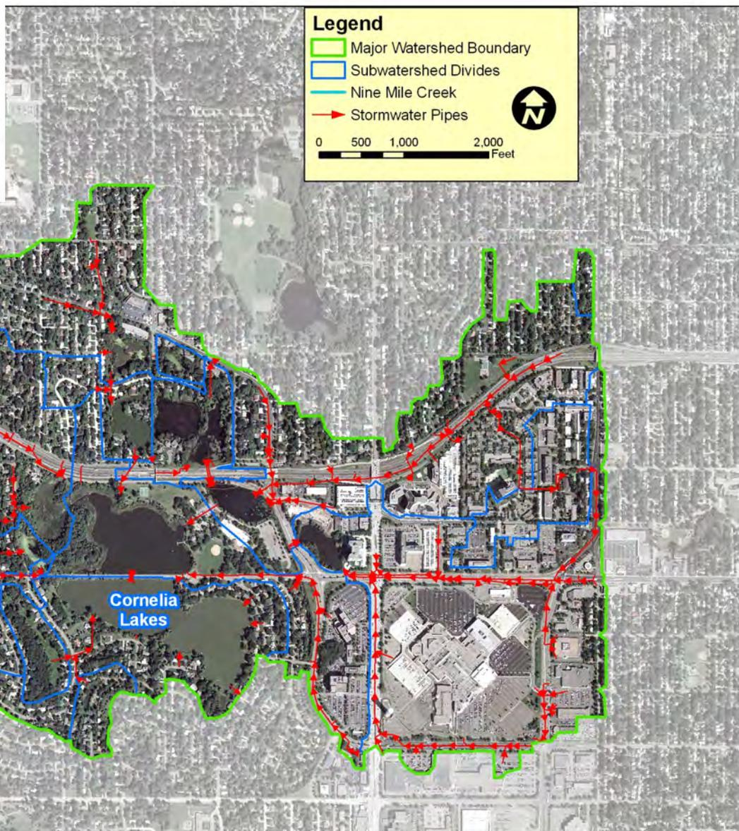
As visibly shown on the map above, a lot of storm drain pipes lead to Lake Cornelia. These pipes carry water to Lake Cornelia that fall on this part of the watershed and is not infiltrated in the ground. The water that is captured runs off lawns, streets, roof tops and parking lots. It then flows right into Lake Cornelia washing and carrying the pollutants left on that land.
