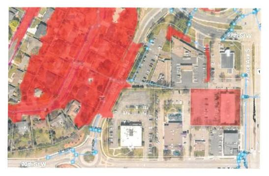
In the interest of incrementally improving this condition, staff has asked the applicant to try to discharge some of the storm water east to the France Avenue storm sewer system. They intend to still control rate and volume with the use of underground tanks and raingardens.
