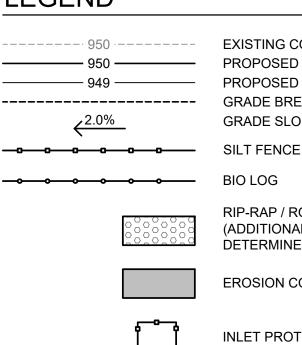
PROPOSED CONTOURS - MAJOR INTERVAL **PROPOSED CONTOURS - MINOR INTERVAL** GRADE BREAK LINE
