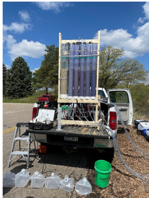
Column testing of filtration media at Rosland Park.
