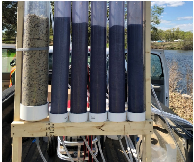
Column testing of filtration media at Rosland Park.
