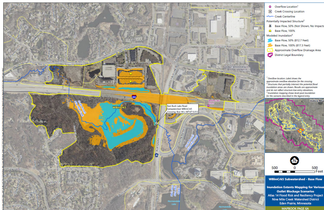
Figure showing results of our detailed crossing failure analysis at the Bush Lake Road crossing. Results show the impact of 50% and 100% failure crossing 10-days after crossing failure during normal baseflow conditions. Results were reviewed recently in response to discovery of a beaver dam in the area restricting flow at this crossing.
