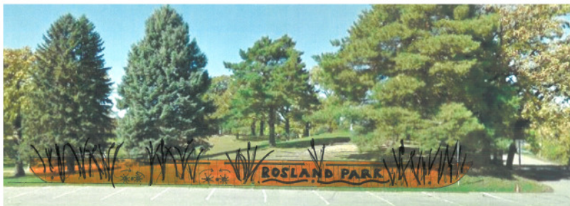
Sketch of preferred BMP concept for a stormwater feature in Rosland Park to treat runoff prior to reaching Lake Cornelia.
