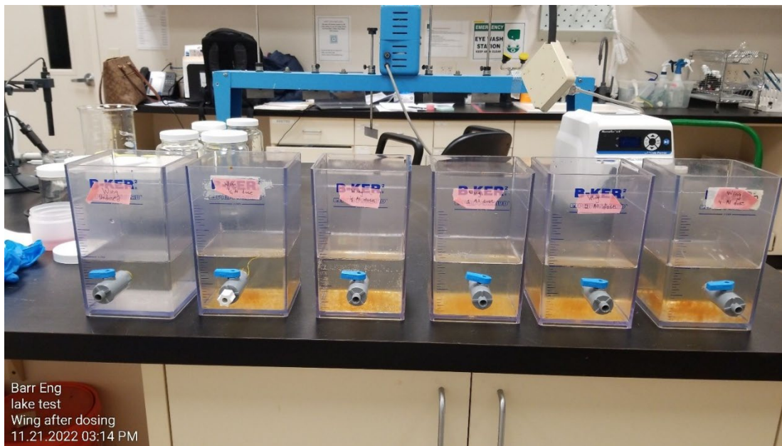
Figure 6-1 Picture of aluminum and iron floc in jar tests with water from Wing Lake treated with ferric chloride and sodium aluminate.
