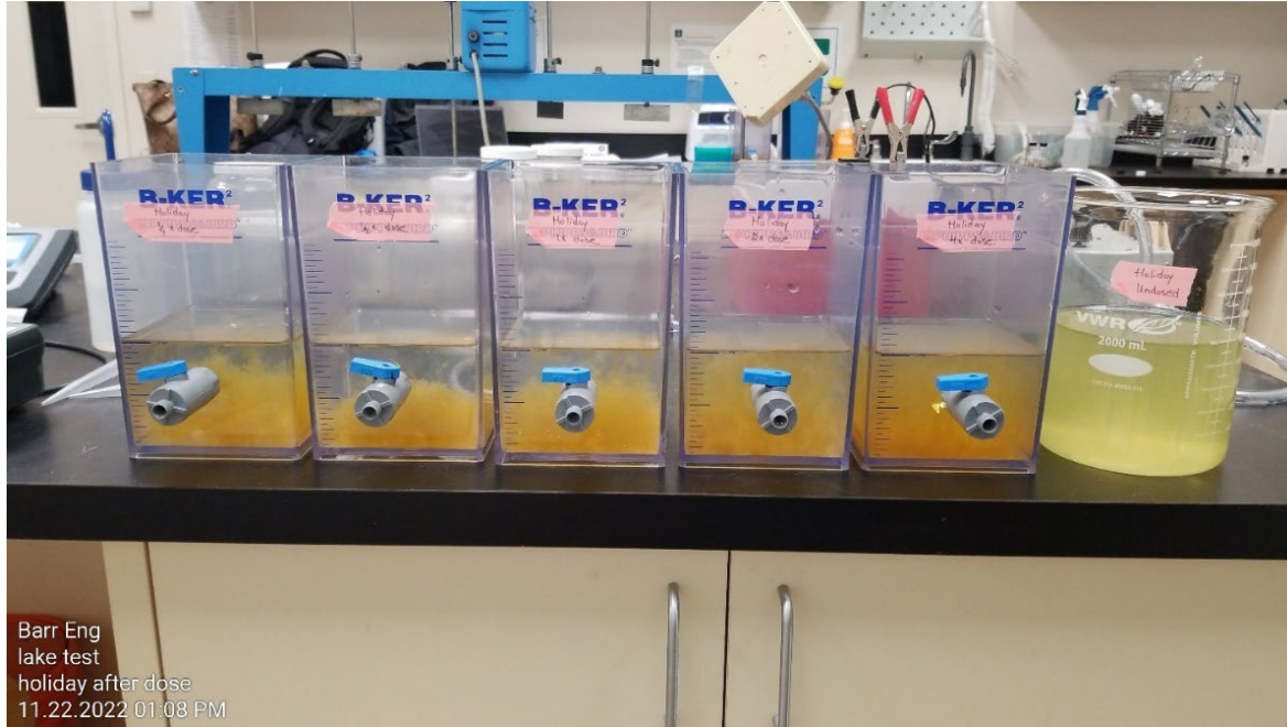
Figure 5-1 Picture of aluminum and iron floc in jar tests with Lake Holiday water treated with ferric chloride and sodium aluminate. (Note that the recommended dosing is the second jar from the left. The far-right jar is untreated Lake Holiday water.)
