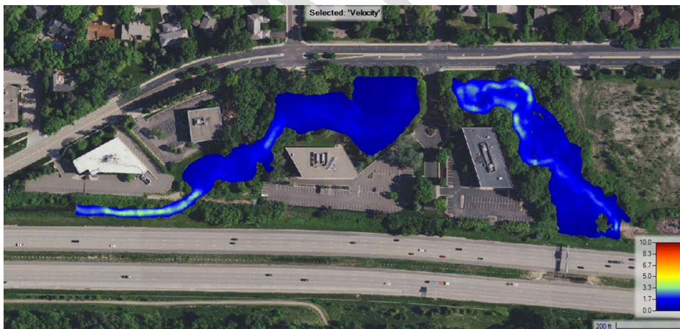
Figure 9. 10-Year Recurrence Interval Flow Velocities (ft/s) for Reaches 16-17
