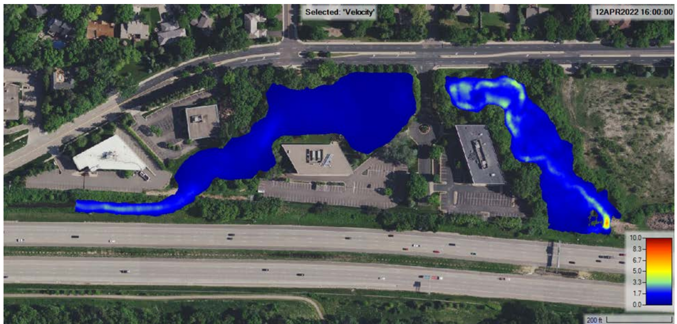
Figure 10. 100-Year Recurrence Interval Flow Velocities (ft/s) for Reaches 16-17
