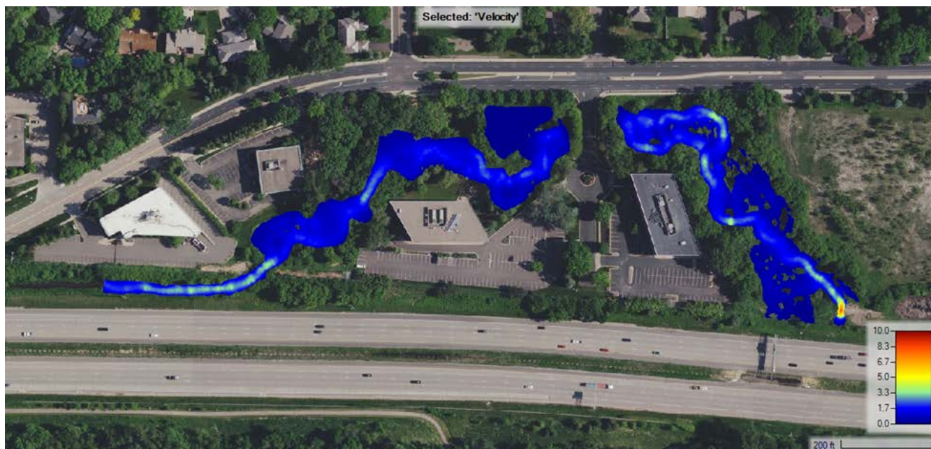
Figure 8. 2-Year Recurrence Interval Flow Velocities (ft/s) for Reaches 16-17
