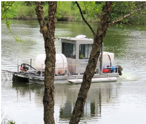
Figure 4-2 Examples of treatment barges that may be used to apply ferric chloride and sodium aluminate to Arrowhead Lake
