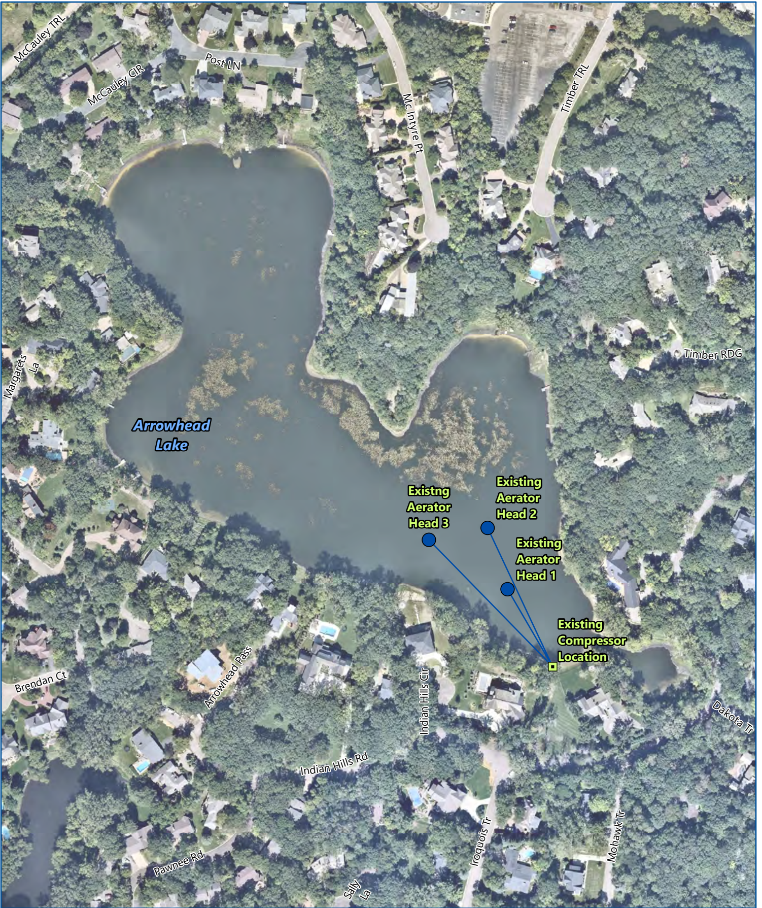
EXISTING AERATOR PLACEMENT Arrowhead Lake Nine Mile Creek Watershed District FIGURE 4-4
