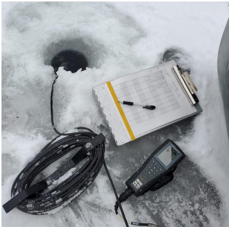
Figure 4: YSI equipment sensing DO at a depth during a winter survey on Indianhead Lake.
