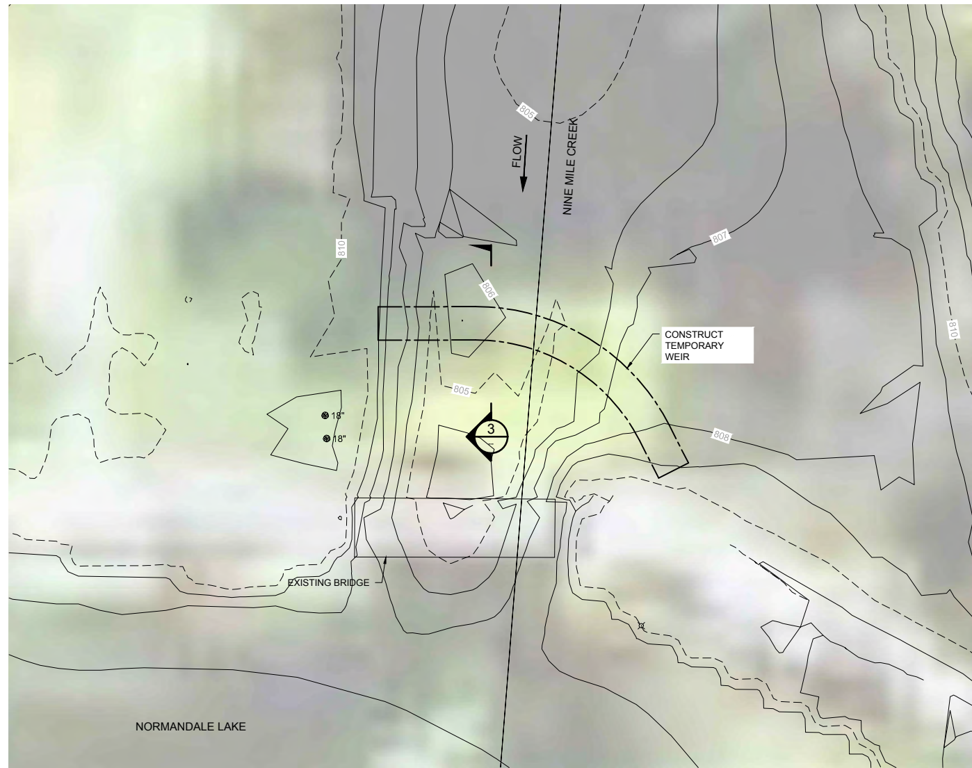
1 PLAN: INLET TEMPORARY WEIR C-01 1"=10' SCALE IN FEET
