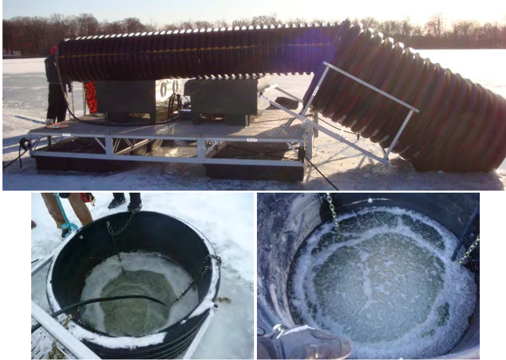
Figure 13: Photos of 24" riser and 48" downcomer being assembled/ deployed (top) and in operation (bottom).
