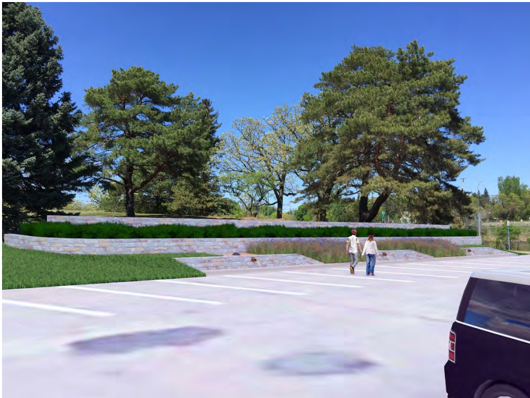
Figure 4-7 Rendering showing the concrete filtration vault with tiered wall planted with shrubs and flowering plants
